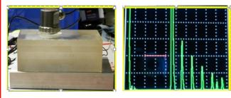
Here we determine the Aluminum equivalent Lucite path distance for the actual 1.9-inch Lucite path distance. The aluminum plate is 1-inch thick. Aluminum velocity is 2.5 X 10^5 IPS; Lucite velocity is 1.07 X 10^5 IPS.
