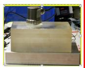
Using a typical A-Scan screen plus the UT test as shown below, let's look at this example of a test with a block of acrylic resin between a contact transducer and an aluminum plate UT inspected with a normal incident transducer on the surface of the acrylic resin.
